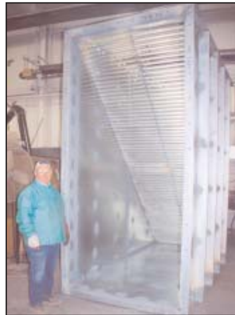
Limbach employee Charlie Mack stands next to the 144-inch-by-72-inch square throat supply air elbow rated at 10-inch wg. with turning vanes.
