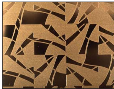
Figure 5: Etched and ceramic-coated stainless steel. Photo courtesy of the Specialty Steel Industry of North America.
