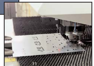
The Trumpf punch press performs intricate, accurate cutting.
