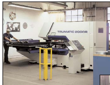
The Trumpf punch press enhances the production at the Budde shop by performing up to 900 hits per minute.
