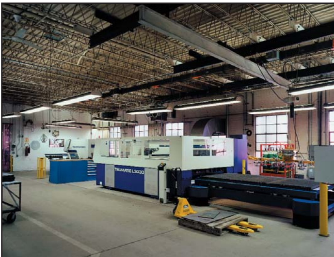
The Trumpf laser cutting center, installed in the Budde Sheet Metal Works shop in 2000, features a 60-inch by 120-inch flat sheet pallet changer.
