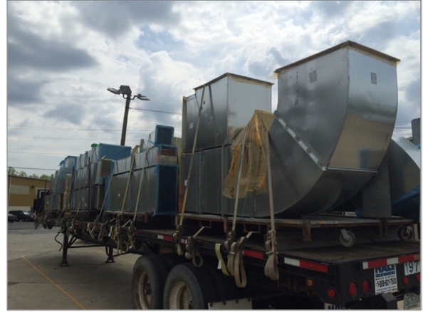
Figure 1: a) Sheetmetal Assemblies Are Ready to Be Shipped, and b) Components Are Ready to Be Assembled in a Shop.
