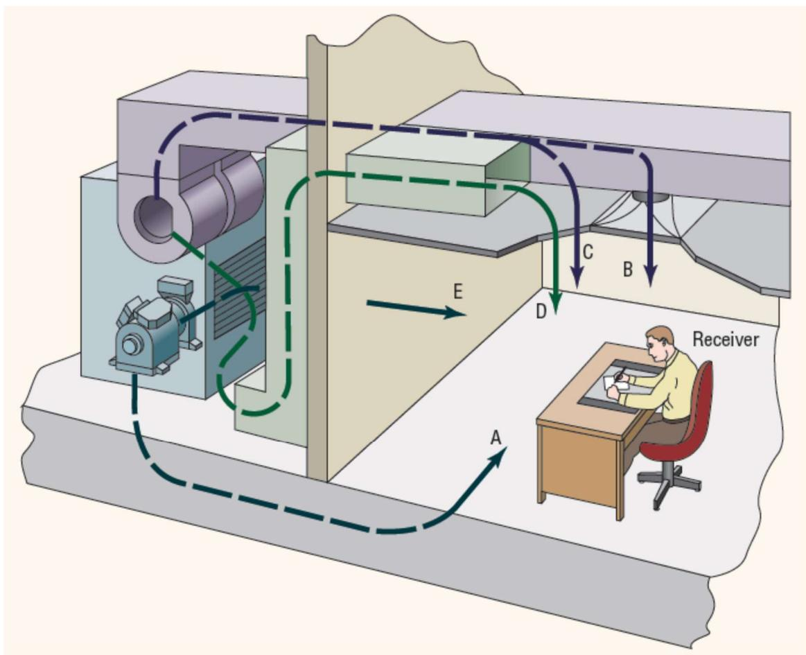
Although there are many different sounds that a receiver (the human) may hear, usually the loudest sound is from the fan. Air movement through ducts also generates noise that travels down the sound path in the ductwork. The ductwork, both supply and return, is generally the main path for the sound (although, as you can see, there are other paths). Metal ducts are very good transmitters of sound. Without proper attenuation, these sounds can be unacceptable at the receiver.
